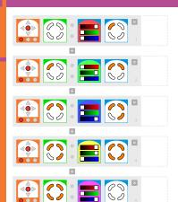
The states allow you to perform different things with the same event, which in this case, is the same button. The green state block defines the state in which the robot can perform the corresponding actions; it's a condition. The blue state block defines the new state after the event; it's an action.
