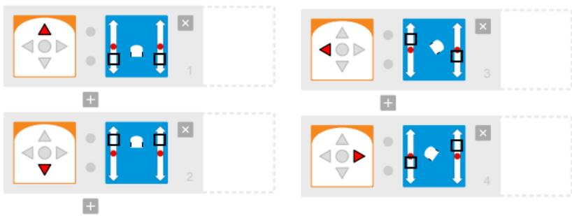
If you set both motors to the same speed, Thymio will go straight either forward or backward. If the speeds are different, the robot will turn.
