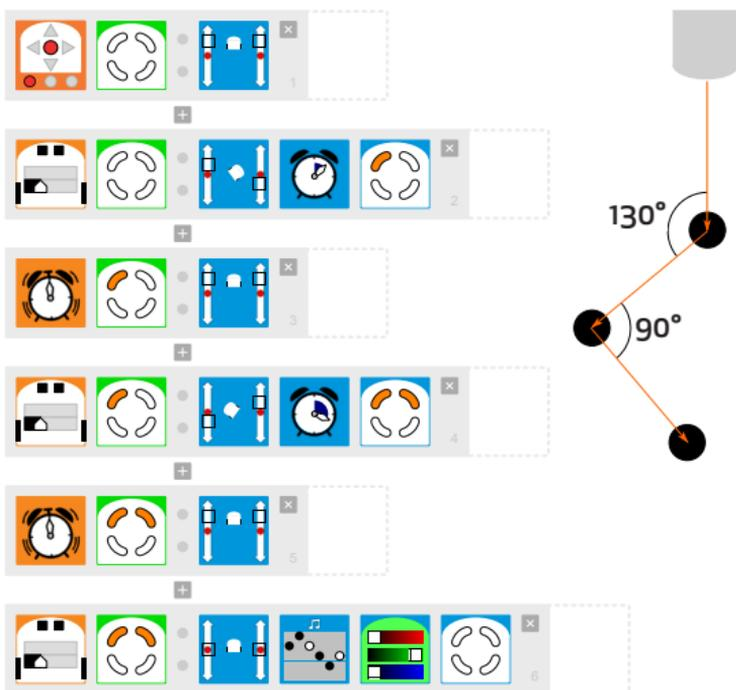
Thymio can detect the targets using its ground sensors. When it arrives at a target, you need to program it so that it turns and aligns itself with the next target, which it can reach by moving forward. Adjust the rotation speed or duration to be as precise as possible.
