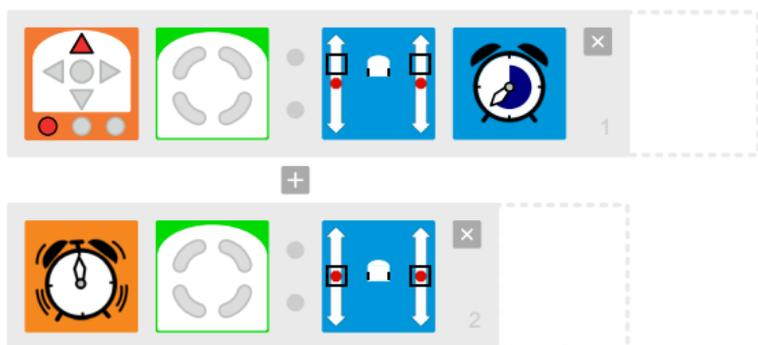
When you press forward, Thymio moves for two and a half seconds. When the time is up, it stops. Adjust the speed and time so that Thymio hits the target! Check to see where it stopped by placing a pen in the pen hole of Thymio.
