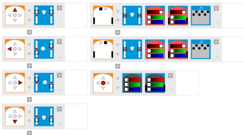
If you program one line for the left ground sensor and one for the right, Thymio will react if it senses something on the left or on the right. With only one block and two black sensors, Thymio should completely cross the black line before lighting up and making noise!
