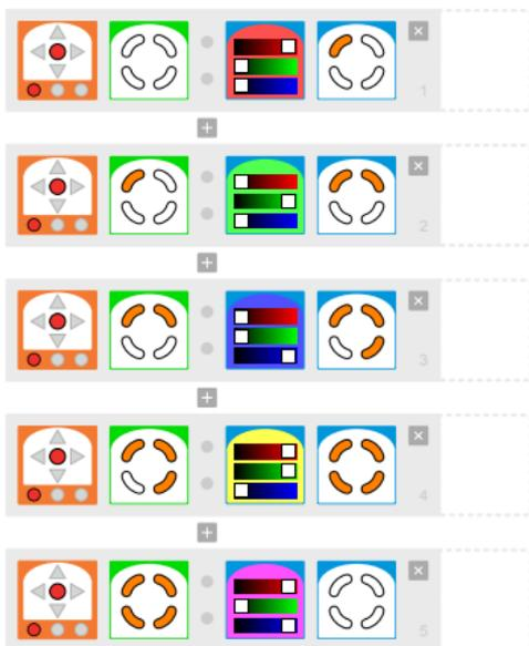
The states allow you to perform different things with the same event, which in this case, is the same button. The green state block defines the state in which the robot can perform the corresponding actions; it's a condition. The blue state block defines the new state after the event; it's an action.
